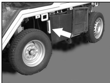
Oil inspection glass
